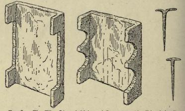
FIG. 85.—Flue-Tiles, Llantwit Major and Caerwent. Also T-headed nails for securing flue-tiles to walls. (All 1/2.)
