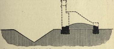
FIG. 15.—Section of Ditch and Rampart, Gellygaer (restoration of rampart in broken lines). (15 ft. to I in.)
