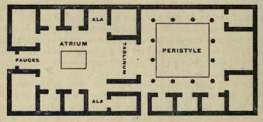
FIG. 40.-Typical Plan of Pompeian House. (After Mau.)
