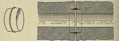
FIG. 86.—Iron Joint for Tree-Pipe, and section showing its use. (1.)
