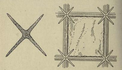
FIG. 81.—Cruciform Iron Object (‡), and its probable use for holding window-glass in its frame.
