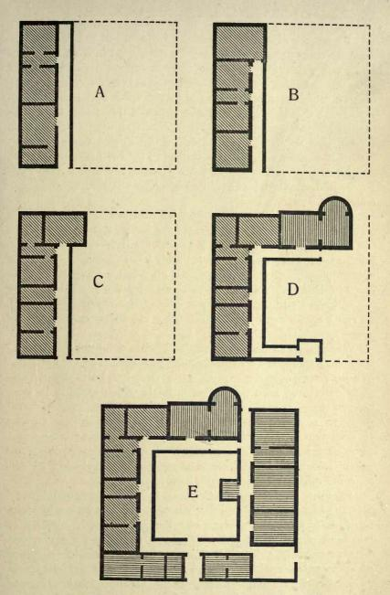
FIG. 41.—Diagrammatic Plans to illustrate the development of the Romano-British House
