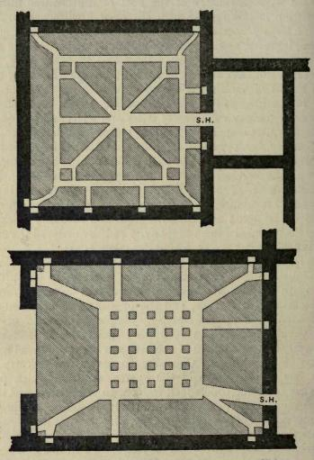
FIG. 82.—Plans of Channelled and Composite Hypocausts at Silchester. (10 ft. to 1 in.)
